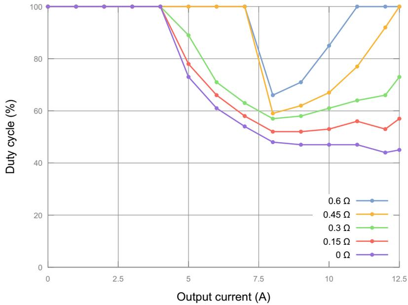
Duty cycle at + 50 °C (+ 122 °F) ambient temperature
