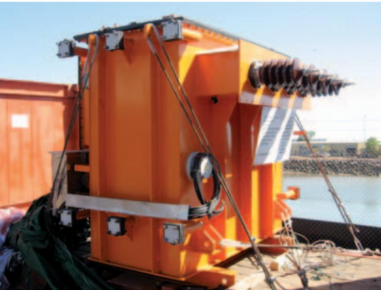
**Singapore—Transformer damaged during shipping:** DIRANA indicated that there was a water content of about 1%. When this was combined with other electrical test results the transformer was found to be electrically sound. A significant amount of water had not spread to the paper insulation.
