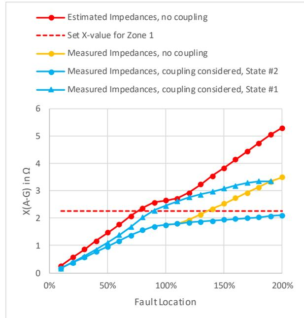
Figure 11: Reactance versus the fault location
