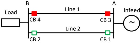
Figure 4: Switching state 3:  $\Delta t_3 = 50\text{ms}$
