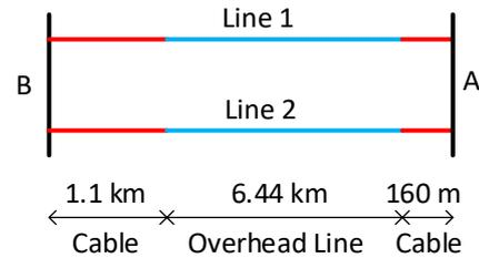
Figure 1: Topology of the double-circuit line
