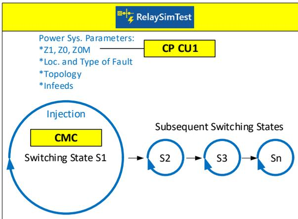
Figure 12: Testing with a predefined sequence of switching states
