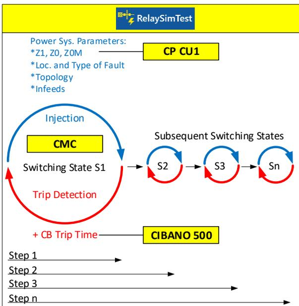
Figure 13: Testing using the “Iterative Closed-Loop” method
