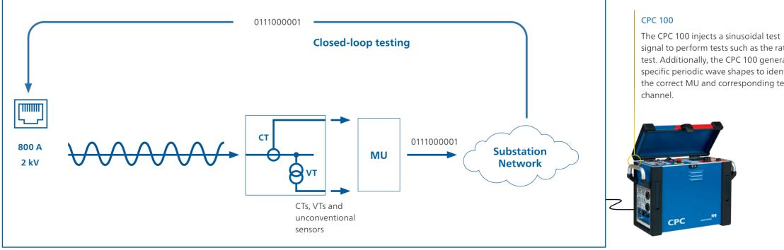
signal to perform tests such as the ratio test. Additionally, the CPC 100 generates specific periodic wave shapes to identify the correct MU and corresponding test
