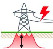
This application module allows you to measure the impedance between the grounding system and reference earth. This type of measurement is also referred to as Ground Potential Rise (GPR), Fall-of-Potential (FoP) or 3-probe-method.
