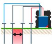
The Soil Resistivity Test (SRT) is performed prior to the construction of a grounding system. Based on these test results, the grounding system is designed to meet all the required criteria. It is also referred to as 4-probe-method.
