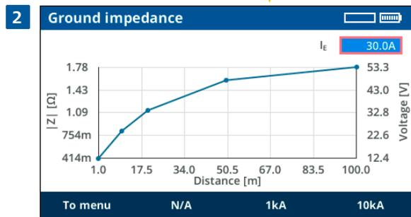
Results can be checked on the display immediately. It is also possible to specify a current to earth to visualize the related ground potential rise directly.
