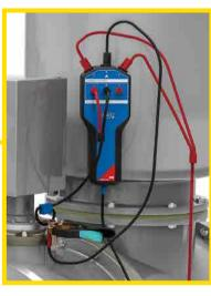
When combined with the new current sensor, CIBANO 500 allows precise timing measurements to be carried out on GIS installations.
