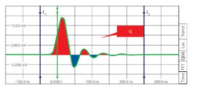
$q = \int_{t_1}^{t_2} i(t) dt = \frac{1}{R} \int_{t_1}^{t_2} u(t) dt$
