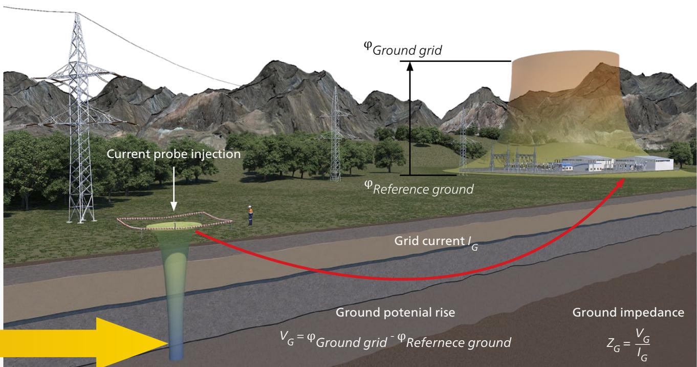
Illustration of current probe injection and ground potential rise
