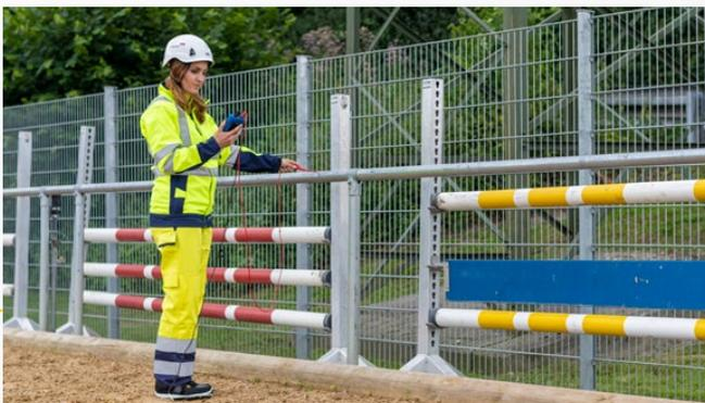
Step- and touch voltage measurement with the handheld meter HGT1
