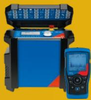
Portable battery-operated primary and secondary injection and basic protection test set. Supports Ground Impedance, Soil Resistivity and Continuity measurements.
