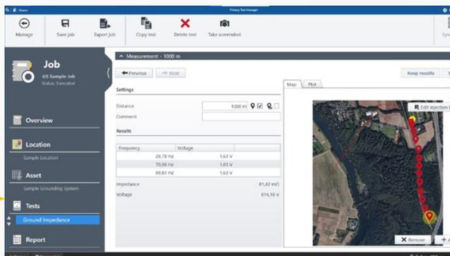
CPC 100: Ground impedance measurement with PTM
