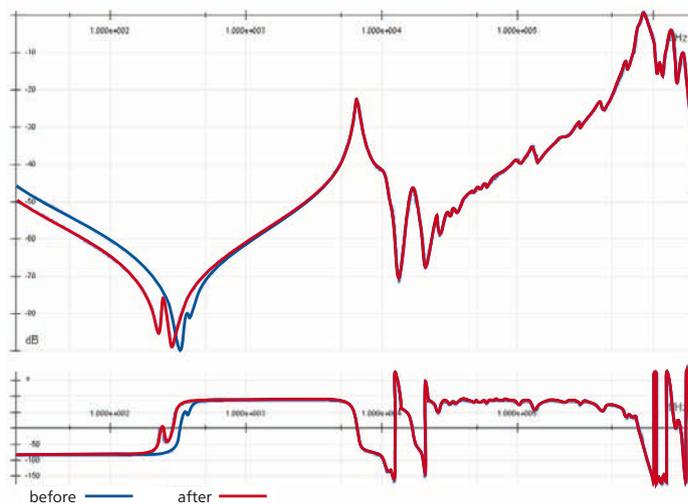
FRA measurement on phase W before and after demagnetization of the iron core.
