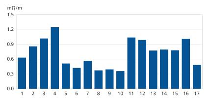
Figure 3: The diagram shows the resistances of the different test points in relation to the distance between the reference point and test point.
