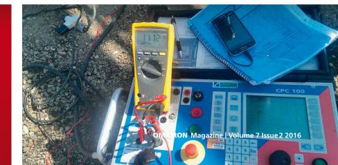
300 A DC that was required, a DC voltmeter, a DC clamp ammeter and markers for identifying the test points (Figure 2). The resistances per meter were determined for several test points in the substation as shown in figure 3. The measurement showed no significant deviations between the relative resistances within the substation. All of the values were between  $0.4 \text{ m}\Omega/\text{m}$ and  $1.2 \text{ m}\Omega/\text{m}$ .
