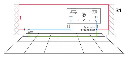
Resistivity, Ground Impedance, and Earth Surface Potentials of a Grounding System" (IEEE 81 standard) different methods for measuring the continuity are mentioned. A 230 kV substation was examined using the 'high-current test method'.
