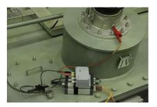
Figure 4 Connection example to bushing
