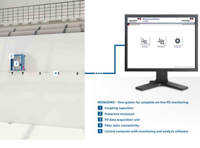
defects that could lead to serious damage and failure in rotating machines," he warns. To indicate increased PD activity, the monitoring software also provides operators with an event log that displays warnings and alarms when PD activity reaches or exceeds pre-defined threshold values.
