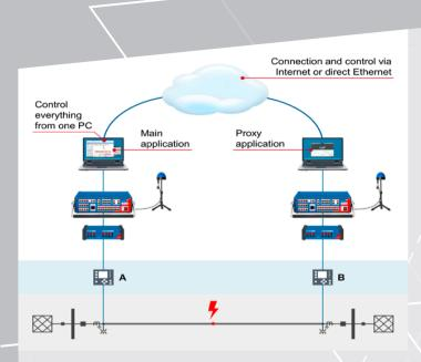
In summation, testing traveling-wave-based relays does not require a new test set, just the TWX1 accessory to expand the scope of your CMC and you are fully prepared, even for the next generation of protection relays.
