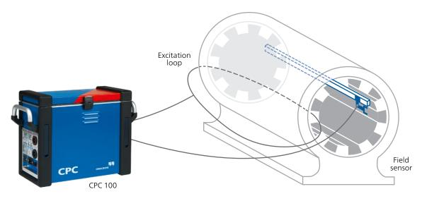
Figure 3. Test setup for a stator core imperfection detection test
