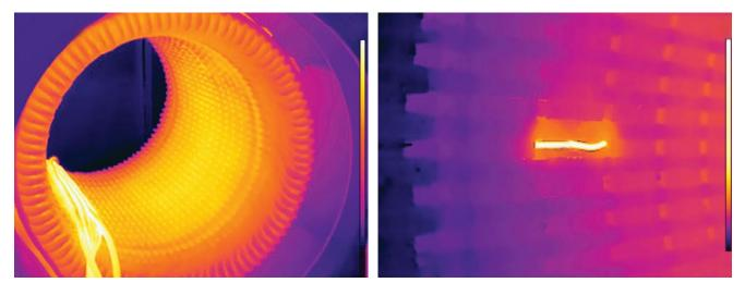
Figure 1: Left: Thermographic imaging during a ring flux test on a small motor. The current in the excitation wires is heating them up. Right: A simulated fault during the test.
