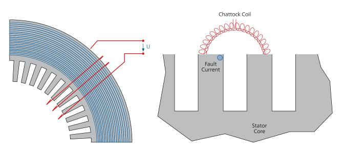
Figure 2: Left: Auxiliary winding and flux distribution within the stator core. Right: Faults are detected by a higher stray flux which is measured with a Chattock coil.
